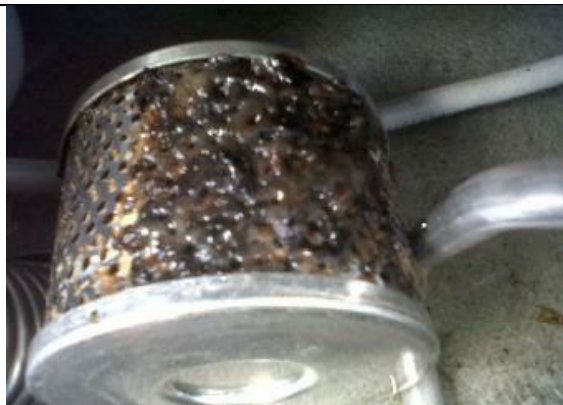
Fuel filter blocked with microbial contamination
