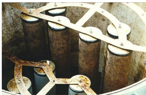
Heavily contaminated filter water separator
