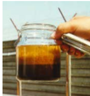
Microbes in fuel samples and found during tank draining.
