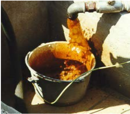
Microbes in fuel samples and found during tank draining.
