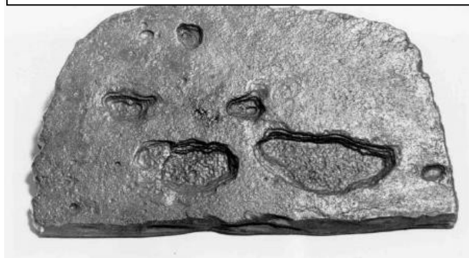
Corrosion pitting in a tank floor plate
